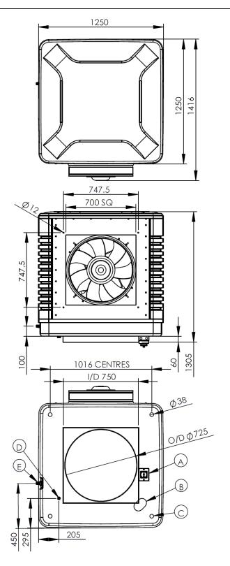
Note that all dimensions shown are nominal and have a  $\pm 10$ mm tolerance due to manufacturing processes employed.
