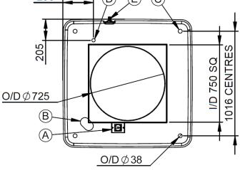
Note that all dimensions shown are nominal and have a  $\pm 10$ mm tolerance due to manufacturing processes employed.
