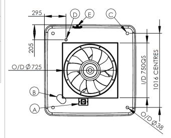
Note that all dimensions shown are nominal and have a  $\pm 10 \text{mm}$ tolerance due to manufacturing processes employed.
