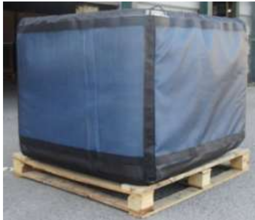
Figure 35. A 4 sided air filter installed on a standard ECPD EcoCooler.
