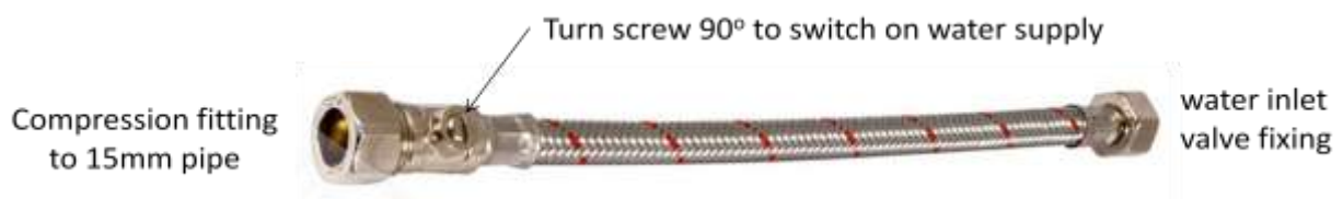
Figure 6. The flexible braided hose with integral isolation valve and 15mm compression fittings, delivered inside the cooler.
