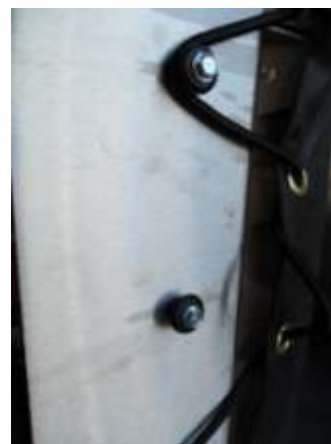
Figures 36 and 37. Installation of a 3 sided air filter on an ECPS EcoCooler. The fastening pegs are located at 11cm intervals, 5cm in from the edge of the fan transmission element, on both sides.
