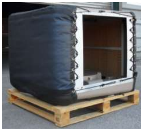
Figures 36 and 37. Installation of a 3 sided air filter on an ECPS EcoCooler. The fastening pegs are located at 11cm intervals, 5cm in from the edge of the fan transmission element, on both sides.
