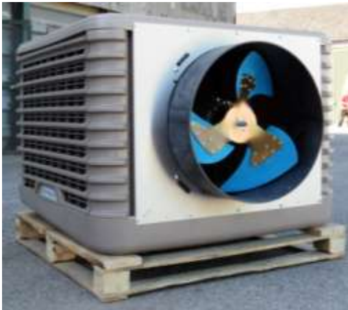
Figures 32 and 33. A 3 bladed fan fitted in a ECPS EcoCooler, and the arrangement of washers for securing.
