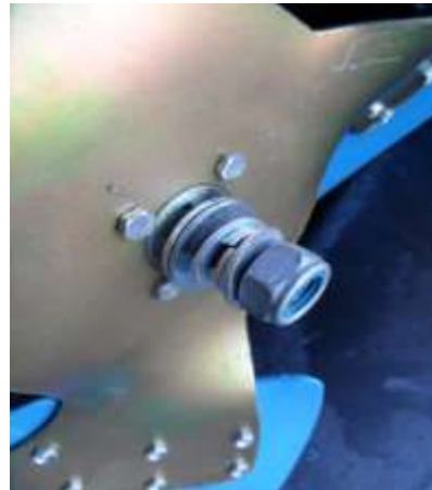
Figures 32 and 33. A 3 bladed fan fitted in a ECPS EcoCooler, and the arrangement of washers for securing.
